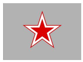
For each complete marking there are 2 masks involved. One is for the main Red star which is applied first, and the second is for the white inset border.
